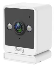
P2-2MP is an indoor infrared camera developed by our company, with 2MP HD image quality, supporting BT5.0, Wi-Fi network connection, supporting human detection, area vigilance, motion detection, infrared night vision. It can be applied to indoor monitoring places such as homes, living rooms, shops, and stores.
