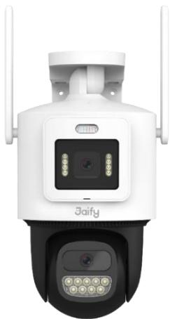
S2-6G-D2 is an outdoor 4G dual-lens PT camera developed by Jaify, with dual-lens design, which can monitor two different areas at the same time, with 3K<sup>+</sup> (6MP) resolution. It features a removable SIM card slot for 4G network connectivity, supporting human detection, human tracking, regional vigilance, dual-light alert, and full-color night vision. IP66-rated waterproof and dustproof for outdoor use. It is suitable for family outdoor, villas, parks, scenic spots, parking lots.
